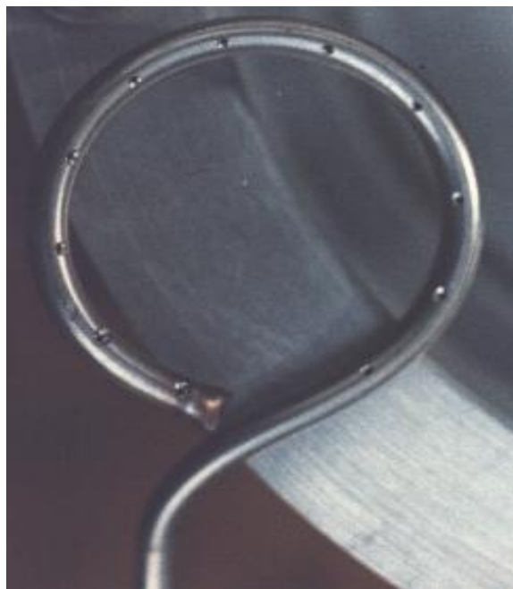
Figure 34 Gas (water vapor) Feed-Ring Electrode Inside diameter of Feed-Ring is 2.78 cm (1.094 inches). Tubing outside diameter 0.318 cm (0.125 inches).
