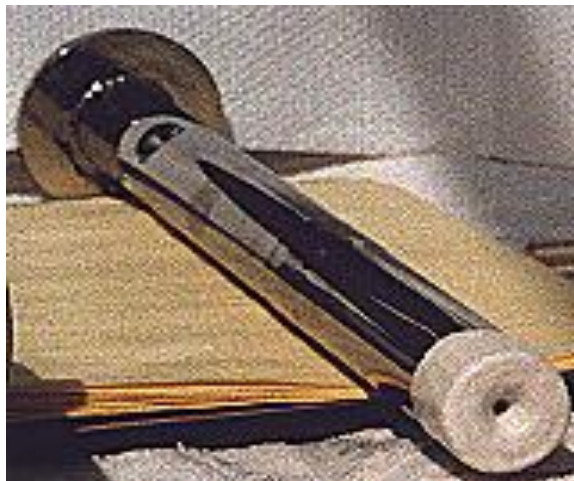
Figure 33 Sonic Quartz Dissociator-Nozzle with Ceramic Zirconia Coating
