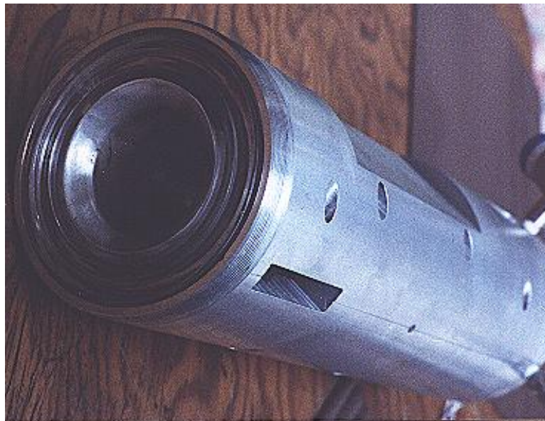
Figure 31 Reactor Containment Vessel
